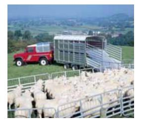
With the deck system folded away the trailer is suitable for use with cattle and other livestock. All components are stored on board the trailer and are conveniently and safely stowed for quick access. When required the deck can be deployed or stowed within a few minutes without the need for any tools or special equipment.
