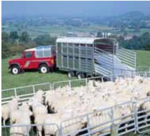
With the deck system folded away the trailer is suitable for use with cattle and other livestock. All components are stored on board the trailer and are conveniently and safely stowed for quick access. When required the deck can be deployed or stowed within a few minutes without the need for any tools or special equipment.
