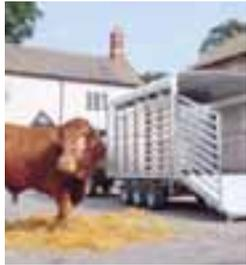
Body lengths of 10', 12' and 14' are available, all with standard headroom of 6'. A tri-axle is an option on the 12' model and standard on the 14' version.
