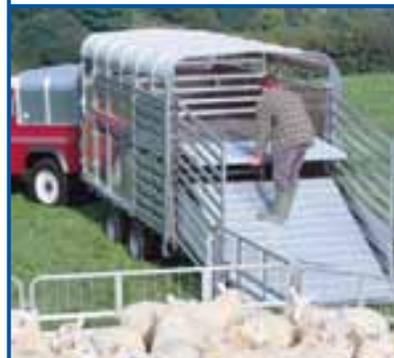
EasyLoad™ deployed and rear barrier lowered.
